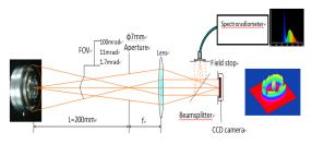
Figure 2 Principle of the measurement system.
